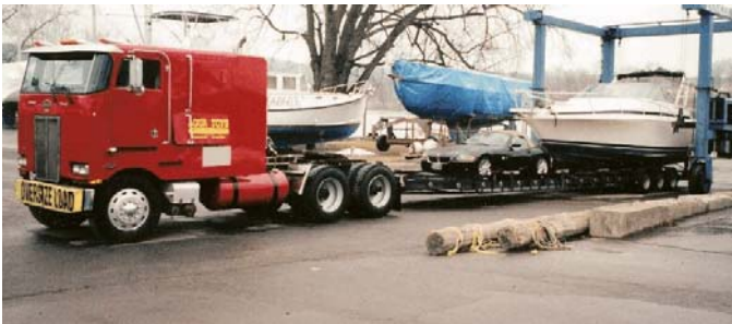
TABT48-213 Tagalong Auto/Boat Transport 48' Long, 21,000 GVWR, Tri-axle
