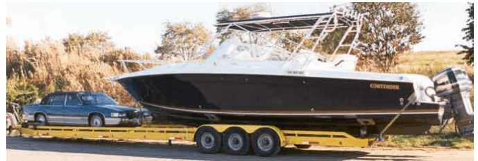
TABT53-243 Tagalong Auto/Boat Transport 53' Long, 24,000lb GVWR, Tri-axle
