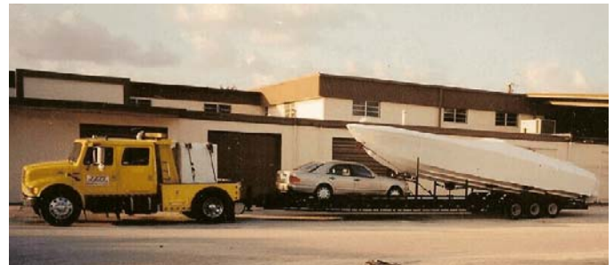
TABT48-213 Tagalong Auto/Boat Transport 48' Long, 21,000 GVWR, Tri-axle Shown with optional Boat Rack
