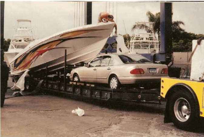
TABT48-213 Tagalong Auto/Boat Transport 48' Long, 21,000 GVWR, Tri-axle Shown with optional Boat Rack
