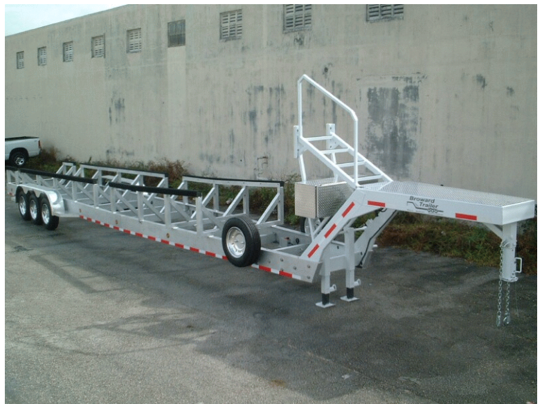
Aluminum Main Frame / Steel Gooseneck
