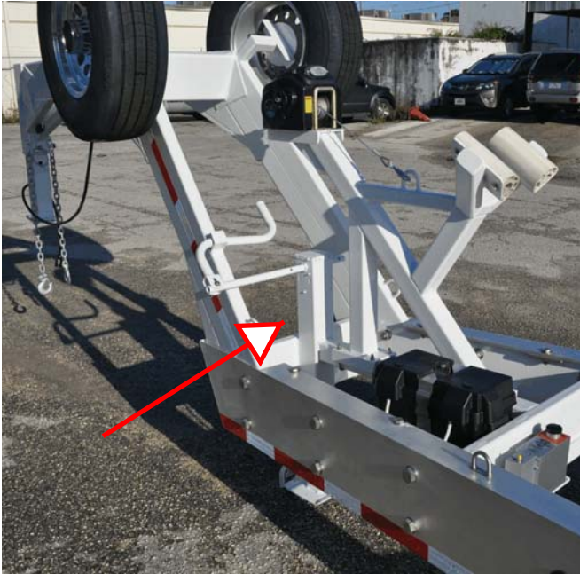
Manual Jack 2 Speed on 30K trailers
